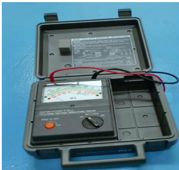
HIGH VOLTAGE INSULATION TESTER / INSULATION VOLTAGE : 5000 V 0 ~ 200.000 M ohm
