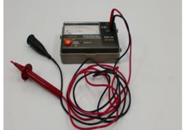
MERGER / INSULATION TESTER VOLTAGE : 500 V 0 ~ 1000 M ohm
