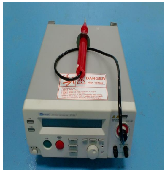
AC / DC WITH STAND VOLTAGE TESTER VOLTAGE : 0 ~ 5 KV AC MAX VOLTAGE : 0 ~ 6 KV DC MAX
