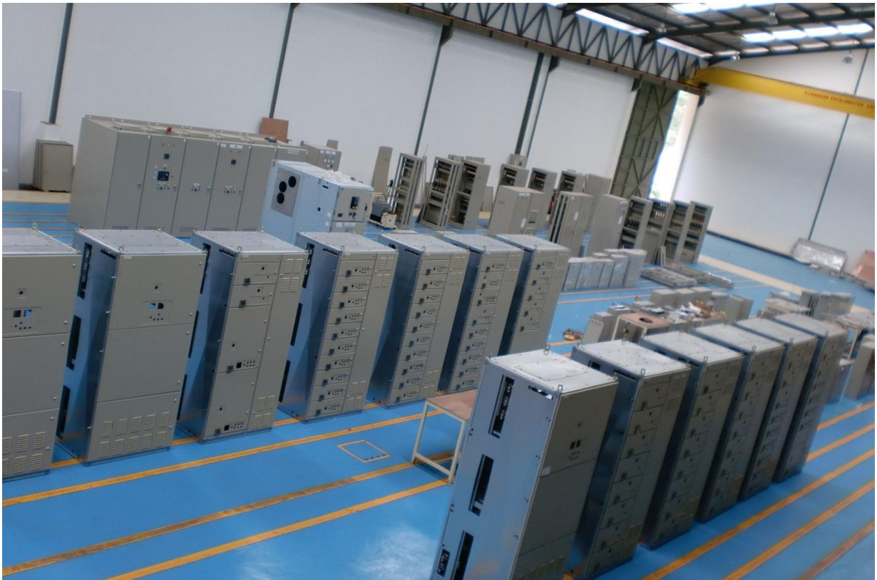
GE SENPlus 400V Motor Control Center Fully Drawout Type
