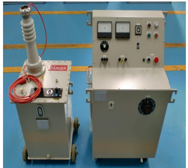
WITH STAND HIGH VOLTAGE TEST VOLTAGE : 0 ~ 50 KV
