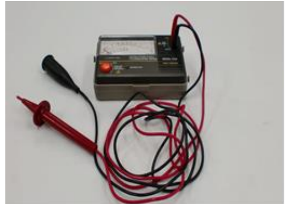
MERGER / INSULATION TESTER VOLTAGE : 500 V 0 ~ 1000 M ohm
