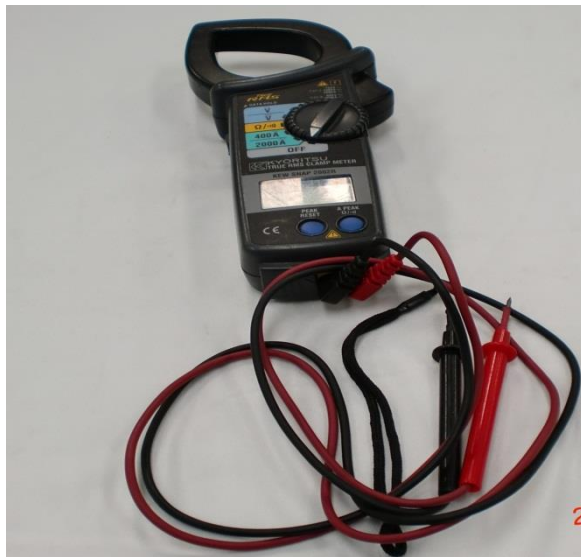
TRUE RMS CLAMP METER VOLTAGE : 0 ~ 1000 V CURRENT : 0 ~ 2000 A
